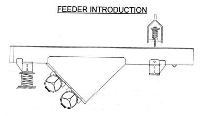
The Vibrating Feeder is a rugged device designed to transfer by means of controlled <u>straight-line</u> vibrations. Stroke, frequency and attack angle combine to pitch and catch conveyed product while moving it horizontally or at a slight incline or decline.
